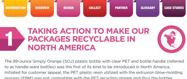
process (EBM) was not compatible with the PET recycling stream and thus the bottles legally had to be coded with #7 (Other) as opposed to #1 (PET) on the bottom of the container. The pressure sensitive labels (PSL) applied on the bottles did not effectively separate during the recycling process.
